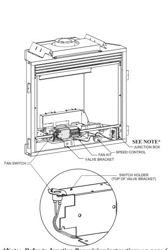
\*Note: Refer to Junction Box wiring instructions on page 68 for proper operation.
